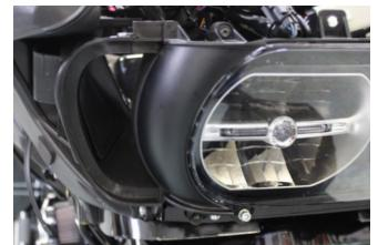
With the outer fairing removed the headlamps, side trim, and side vents are now exposed.
