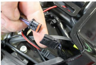
Locate the turn signal wire plugs. They are three wire plugs with a black, purple and blue wire. Unplug both the left and right turn signal plugs.
