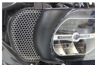
When the vent screens are shaped properly there should be a slight friction fit to hold them in place. If they do not hold themselves in place a couple of dabs of silicone on the top and bottom edges of the screen can hold them in place.
