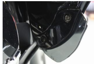
With your T25 Torx driver, remove the screws and wind deflectors located under the left and right glove box doors.
