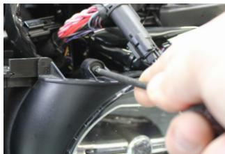
Remove the headlamp left and right side trim pieces with your T25 Torx driver. There is one screw on the top and the bottom of the side trim pieces.
