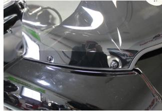
Remove the four phillips screws holding on the windshield. Remove windshield.
