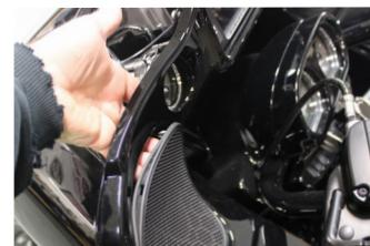
Remove the left and right speaker grill. From the open top side of the fairing you can press on the inside of the speaker grills and pop them out. There are two snap in plastic inserts holding each grill in.
