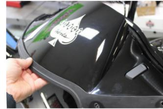
The cowl piece is now free to be pulled away from the inner fairing and removed.
