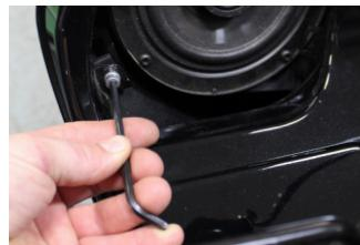
Remove the T27 Torx screws located in the speaker opening of the inner fairing. **Once these bolts are removed your fairing will be loose and no fasteners will be supporting the fairing. You may want assistance from a friend to support the outer fairing during this step.**
