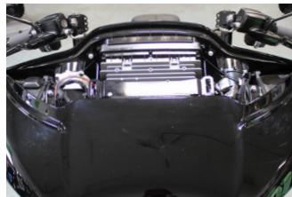
With the cowl removed the top of the radio and speaker pods are exposed.
