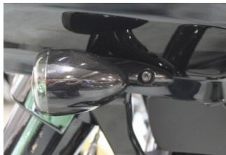
With your 3/16" Allen Wrench remove the bolts located behind the left and right turn signals.
