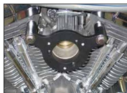
8. Install the K&N® crankcase breather plate along with the two remaining o-rings, mounting bolts (with one drop of thread locker) and the throttle body gasket as shown.
