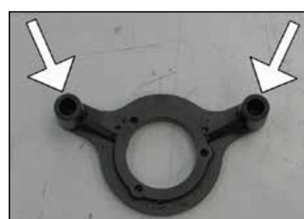
7. Install two of the provided o-rings into the K&N® crankcase breather plate as shown.
