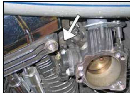
6. Using the provided tie wrap, secure the wiring pig tail to the throttle body wiring harness.
