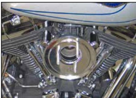
9. Install the three spacer/bolts into the K&N® filter base plate, then install the base plate gasket and one drop of thread locker onto each spacer/bolt. Install the K&N® filter base plate assembly onto the breather plate as shown.
