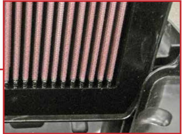
Fig. 2 Filter sitting in groove correctly
