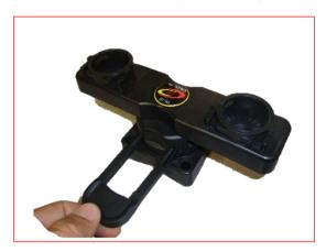
10. Insert the Rhino Grips in the desired position on the doubler plate and secure using the Kwik Clips provided. NOTE: Grip can rotate 360° to accommodate any angle, and the grip can tilt 0° to 180° at 45° increments.
