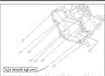
Under racing propose, could remove the box cover to increase the air flow to get better performance. Just tie up all necessary screws as the instruction manual shows.
