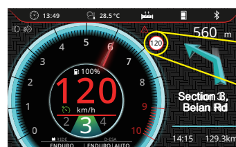
●Navigation screen of the meter.
