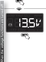
•In the voltage screen, press the button to enter the MAX screen.
