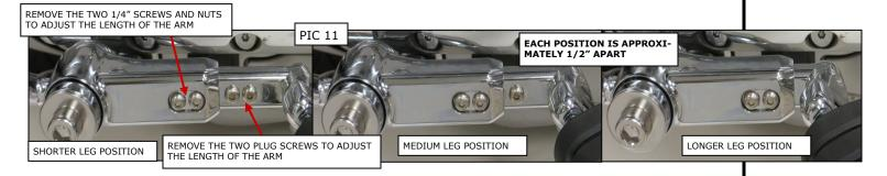
**STEP 21** Confirm that the pegs fit and function properly **BEFORE** riding the motorcycle. The Ergo III Adjustable Cruise Arms **MUST** return on their own when your feet are removed from the pegs.
