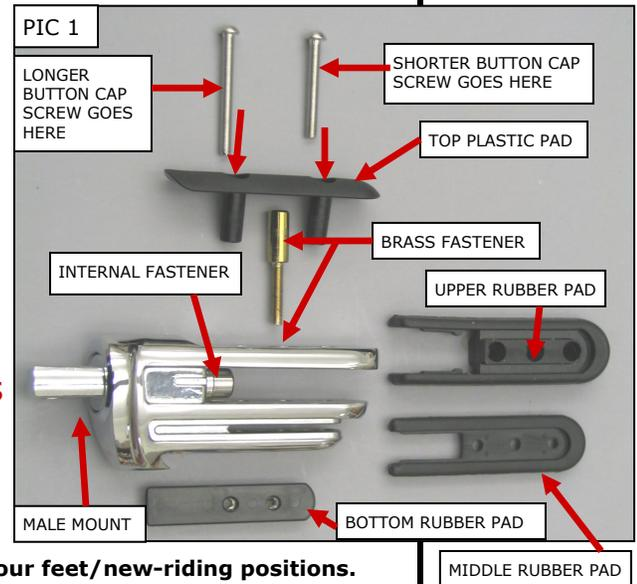
**STEP 10** Tighten all fasteners.
