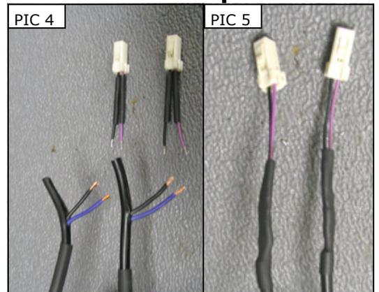
**STEP 6** PIC 5 shows the finished wires after the shrink tube has been installed.
