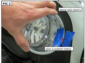
Position the Right Driving Light Bezel as shown in **PIC 3**.
