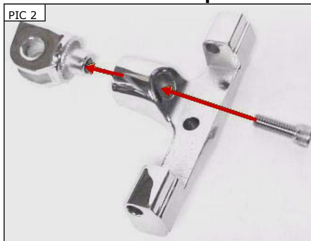
**ATTENTION!** Ensure that the supplied anti-seize is applied to all threaded fasteners before installation; this will make future removal of the fasteners easier.
