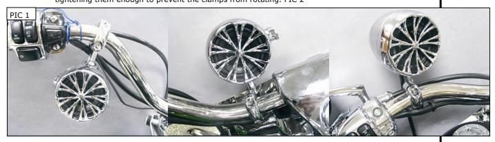
NOTE: The clamps may be installed in different directions/positions as needed for sufficient clearance.
