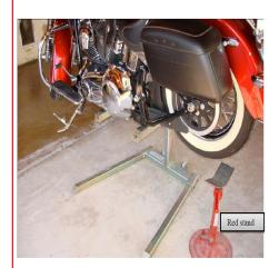
2. Using an 11/16" wrench, remove the shocks front hardware (nut, bushing & cup washer).
