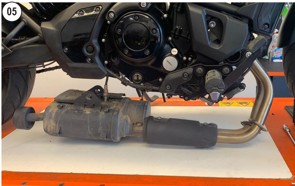
REMOVE THE STOCK EXHAUST
