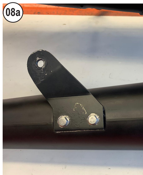
FIT THE LeoVince's BRACKET AT THE MUFFLER
