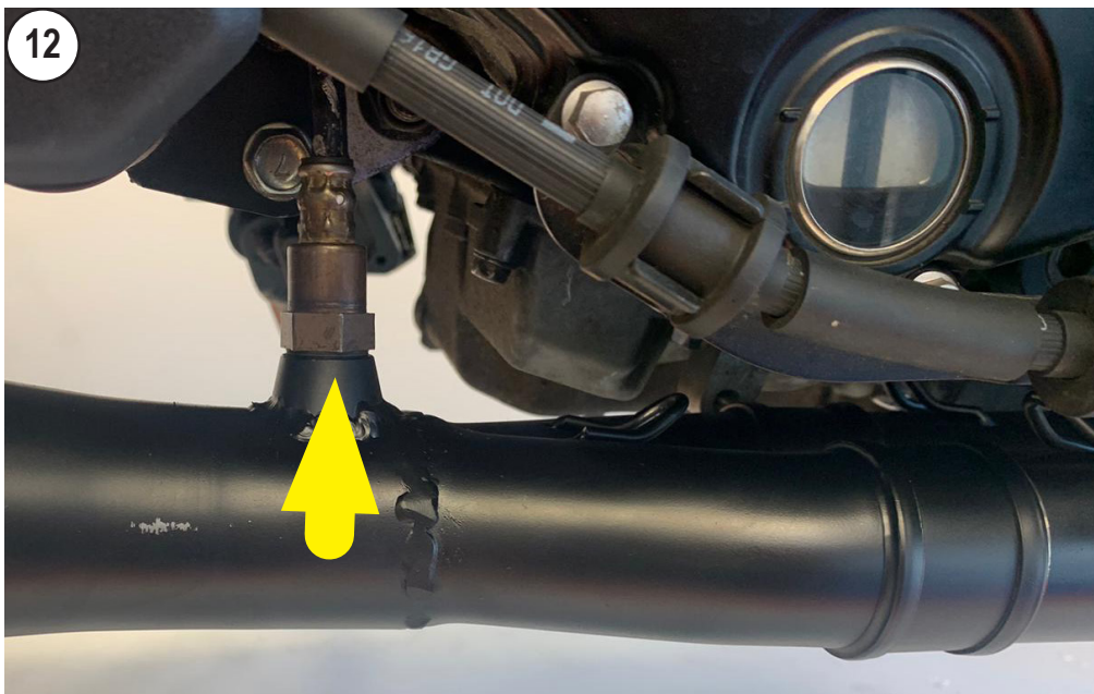
SCREW THE LAMBDA SENSOR
