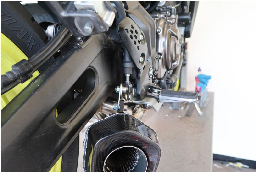
Tighten the 4 x header nuts to 20Nm torque setting.
