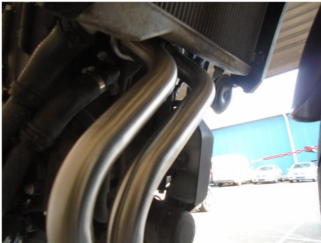
Re-install the Lambda sensor AND brass adaptor ensuring that the specified torques are used.
