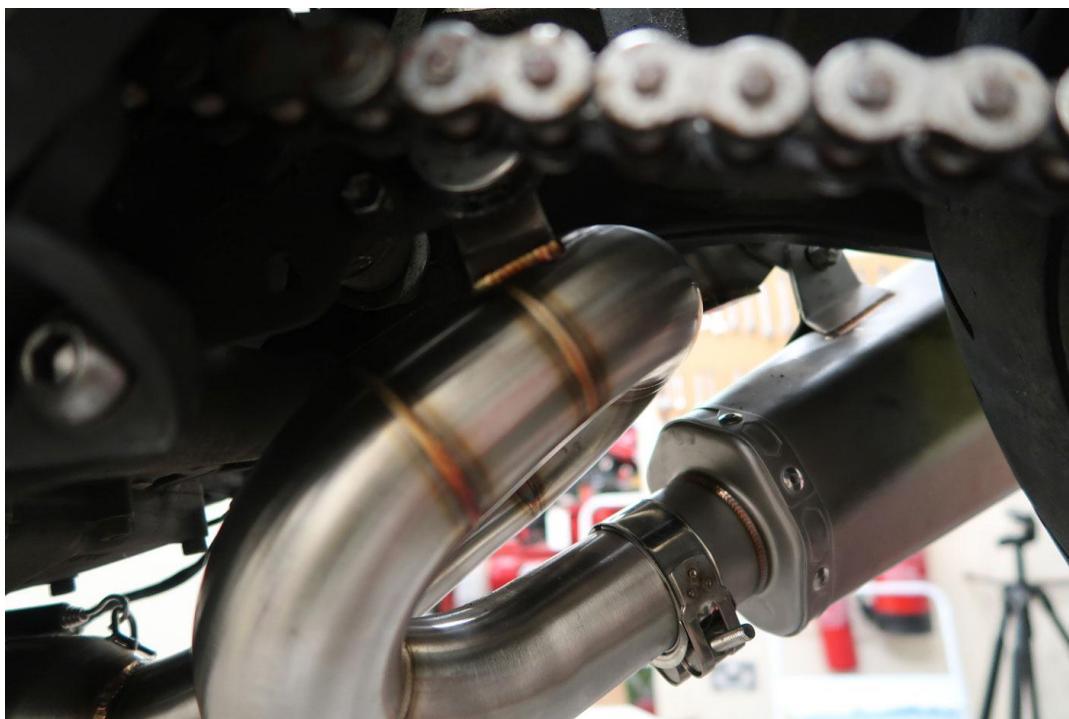
Mount your new Lextek Silencer to the header and line the mounting point on the silencer to bracket (installed earlier). Using the bracket and bolts (supplied) secure the silencer ensuring the correct torque settings are used.
