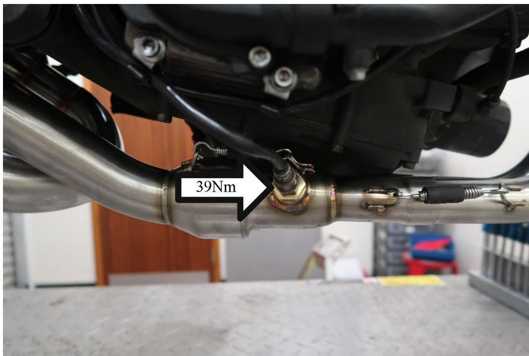
Install the rear section of the exhaust system and secure in place using the retaining springs (supplied).
