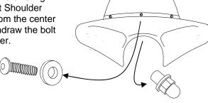
3. Align the Polished Solid Stainless Steel Trim over the center hole and insert a Stainless Steel Button Head Screw . Secure in place with an Acorn Nut Shoulder Spacer
