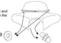
Align the Polished Solid Stainless Steel Trim over the left and right holes and insert Stainless Steel Button Head Screws.
