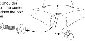
3. Align the Polished Solid Stainless Steel Trim, Slim Style over the center hole and insert a Stainless Steel Button Head Screw . Secure in place with an Acorn Nut Shoulder Spacer
