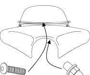
4. Remove the existing Acorn Nut Shoulder Spacers from the left and right holes. Withdraw the bolts and washers.
