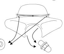
5. Align the Polished Solid Stainless Steel Trim, Slim Style over the left and right holes and insert Stainless Steel Button Head Screws. Secure in place with Acorn Nut Shoulder
