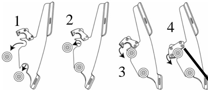
1. Place lower slot into lower bushing. 2. Rotate top slot into place. 3. & 4. Secure locking Mechanism.
