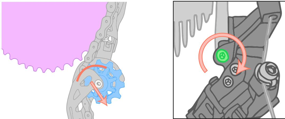
Snap **the derailleur adjustment tool** on to the **guide pulley**. Make sure **the tool** is touching the **chain** but not touching the **cassette cog**. Tighten the B-tension screw if the tool does not have enough room.
