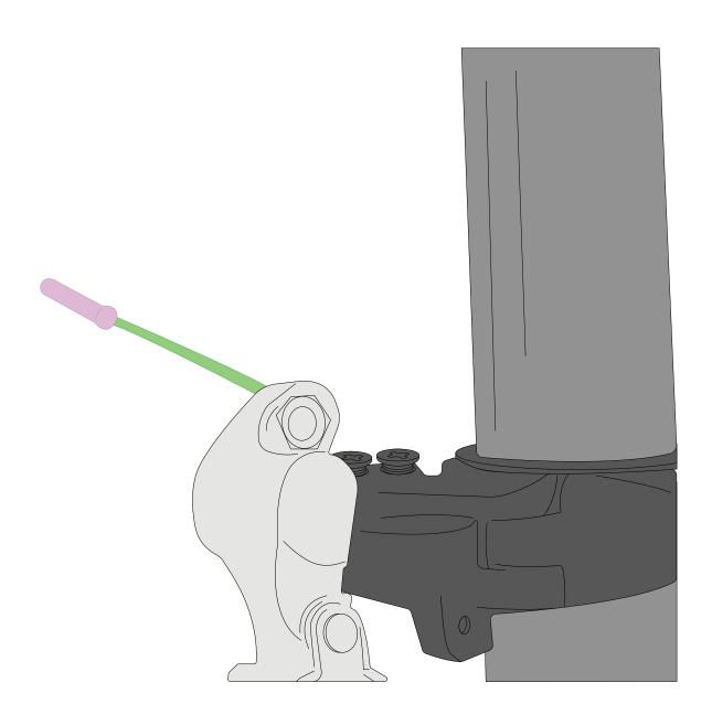
Shift between chainrings. If the **chain** struggles to shift from the largest to smallest chainring, your cable is too tight. If available, turn the **barrel adjuster** on your frame or shifter clockwise. Make incremental adjustments. Test the derailleur for function after each adjustment.
