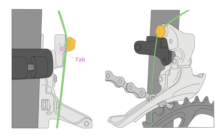
Pull the **cable** tight to remove any slack and secure the cable fixing bolt to **5 - 7nm**.
