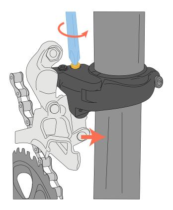
Route your **shift cable** and housing. Every frame manufacturer has a different cable routing guideline, so make sure you consult those first before sizing and cutting your housing. Route the **shift cable** through the housing, over the **tab** and through the **grove** below the **cable fixing bolt and washer**.
