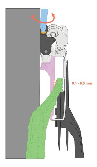
Turning the screw clockwise moves the cage toward the outer chainring, and turning it counterclockwise allows it to move toward the inner chainring.
