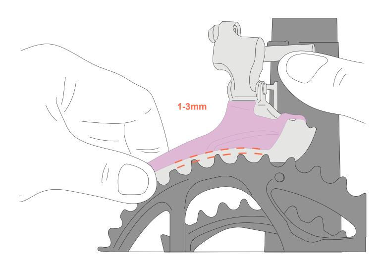
Tighten the mounting bolt with 5mm Hex bit to 5-7Nm.
