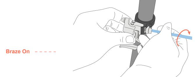
Position the derailleur so that the outer plate of the chain guide is parallel to the largest chainring.
