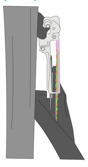
Position the derailleur so there is 1-3mm of distance between the derailleur's outer plate and the largest chainring.
