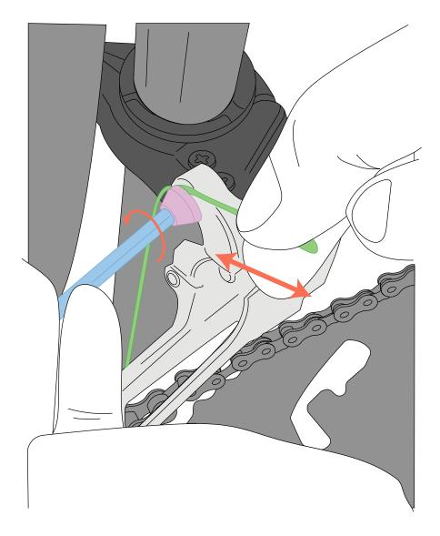
With the chain on the large chainring, shift the **chain** to the smallest cassette cog. This puts the chain at its most outboard possible position.
