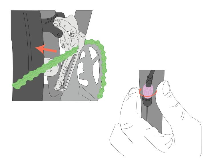
Shift between chainrings. If the **chain** struggles to shift from the smallest to largest chainring, your cable is too loose. If available, turn the **barrel adjuster** on your frame or shifter counterclockwise to increase cable tension. Make incremental adjustments. Test the derailleur for function after each adjustment.
