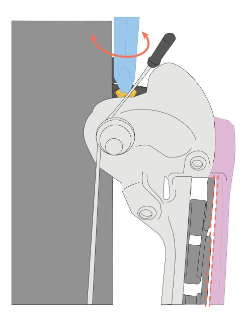
Turning the screw clockwise moves the cage towards the inner chainring. Turning the screw counter clockwise allows the cage to move towards the outer chainring.
