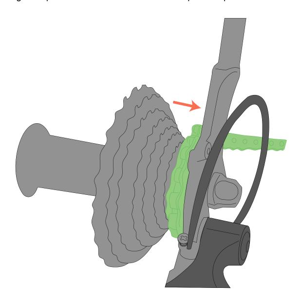
Turn the high limit screw until the gap between the chain and the outer place of the derailleur is about 0.1-.5mm.
