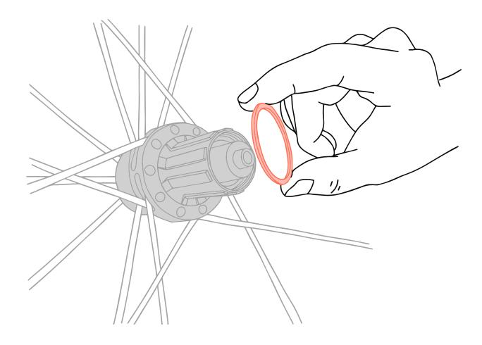
Align the **small spline** on the freehub body with the **small spline recess** on each cassette component, then slide on each component in order as shown in the **Installation Order** section of this manual.
