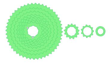
Sword **G-Series** cassettes use two **aluminum spiders** to mount the largest 5 cogs, with smaller cogs and spacers installed individually.
