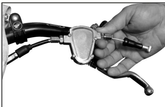
**7 Attach the supplied cable (sticking out of the EZ-pull box) to your clutch lever.**
