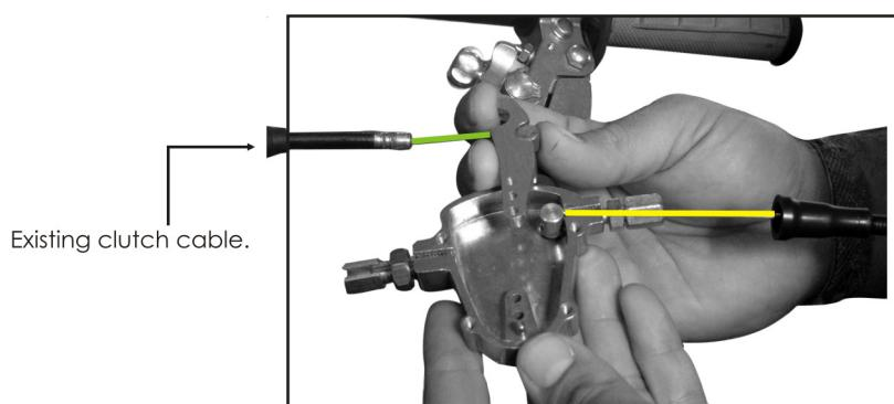
**5 The slot axis will give the greatest increase in leverage.**
