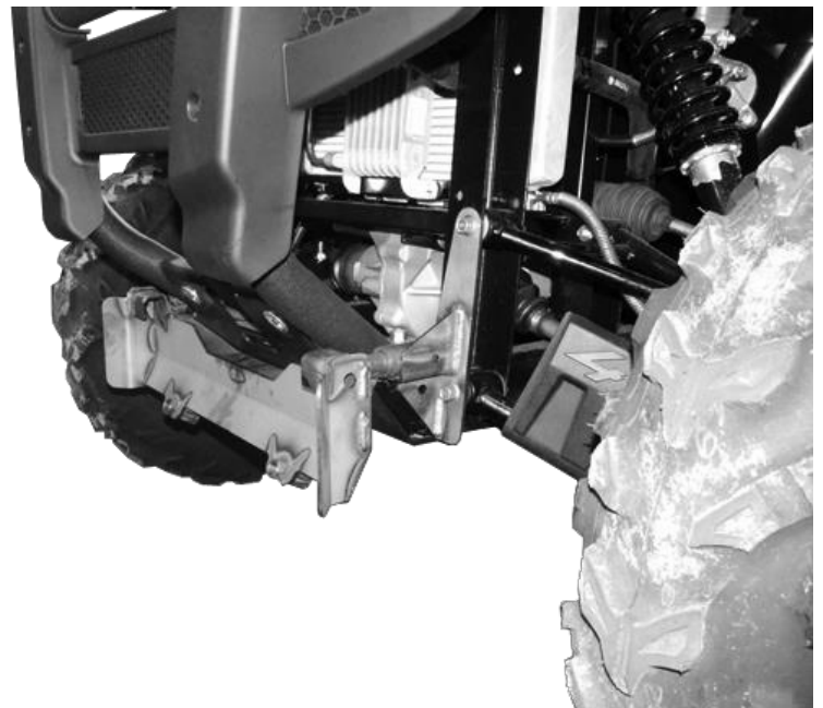
Complete mount system installed on machine.
