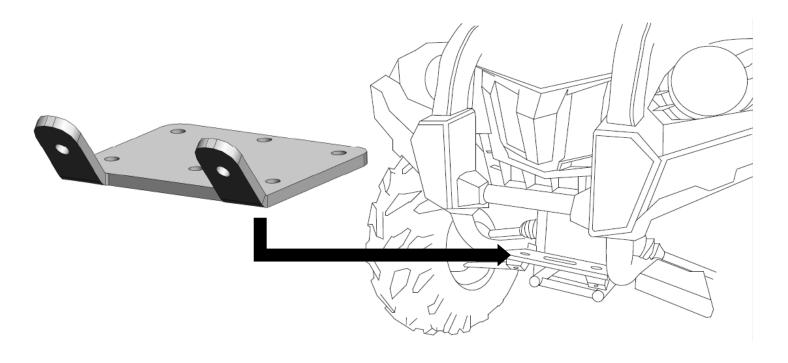
Winch Mount Plate will lay inside front bumper on cross member and go between the winch and the cross member. Bolts will be in the winch kit and will bolt up through the cross member, through the winch plate and into the winch. Bolt fairlead to the front with hardware provided by winch manufacturer and wire to their instructions.
