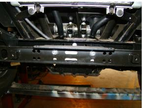
Install winch to winch plate with hardware provided with winch. Next place mount in place on top of support plate and bolt down with  $5/16 \times 1$  hex bolts, four flat washers and nylock nuts. Secure in back with  $3/8 \times 1$  hex bolts, washers and nylock nuts.
