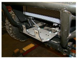
Attach fairlead with hardware provided with the winch.
