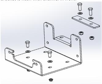
3. Place winch mount in place as illustrated. Attach to angle bracket with two 5/16" x 3/4" hex bolts and wiz nuts, attaching to front cross support. (If bolting winch on this flat surface, the winch bolts will secure winch mount in this location.)
