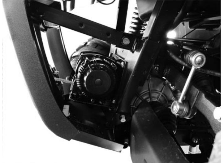
**Position the winch on the mount from the side.**
