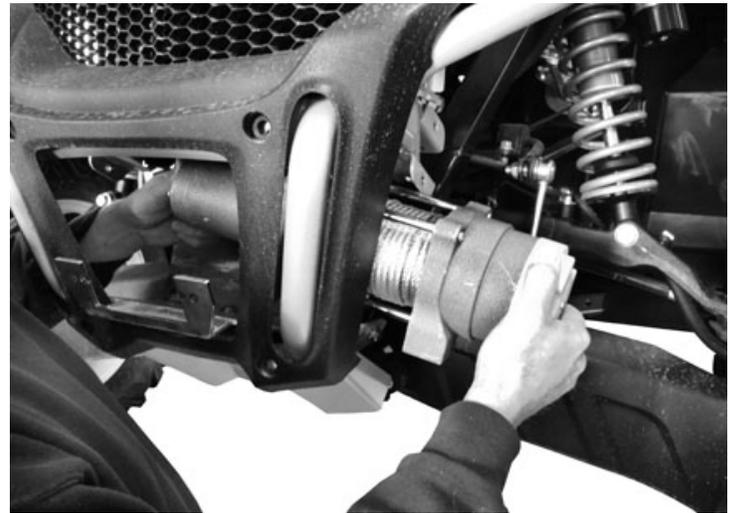
Position the winch on the mount from the side.
