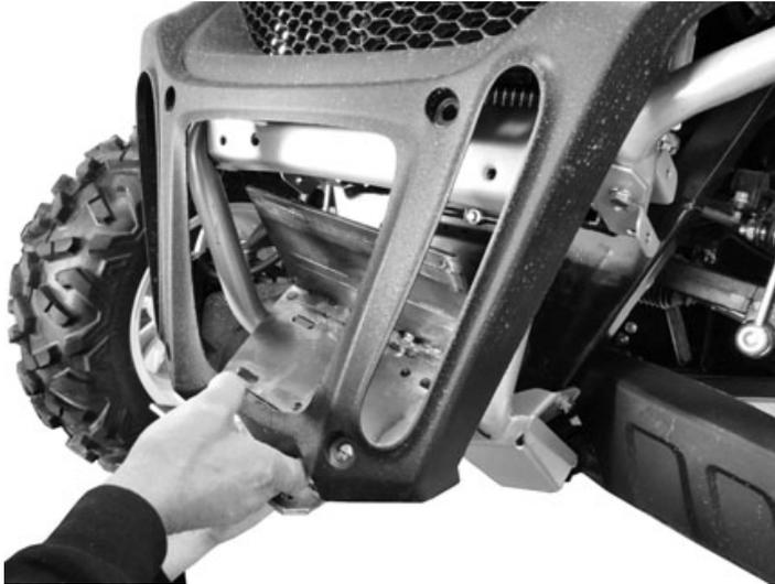
Slide the winch mount into place from the front.
