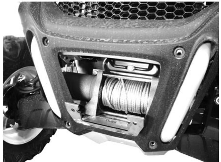
Secure the winch/mount assembly to the frame on the backside using the 3/8" flange nut.
