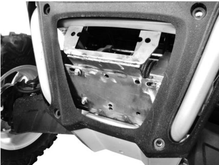
Put the 3/8" x 1" bolts into the back of the plate. Next, rotate the winch and plate up so you can bolt the winch to the winch plate.
