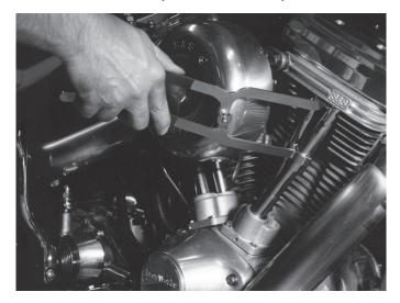
To use the Motion Pro Push Rod Tool, slip the flat portion of the tool under the bottom fin on the head. The cup then goes over the cap or the larger portion of the tube. Compress the handles and the Spring Cap Retainer is easily removed or installed.
