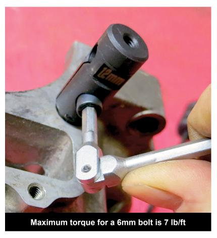
**Step 1:** Select the correct size collet for the dowel pin you are going to remove
