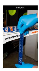
**Note:** Be sure to use the same reference point with each measurement taken. If possible, try to take your measurements with the scale perpendicular to the floor. An angled measurement is not as accurate.
