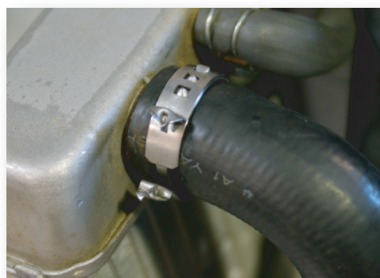
Ready to remove, and not reusable.
