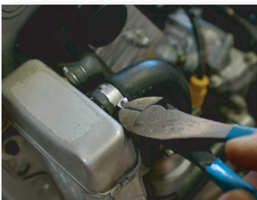
Cutting through the ear of the stepless clamp to remove it
