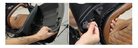
2. Locate the eight bolts mounting the armrest to the trunk. Remove these with a 6mm Allen wrench. This will disconnect the two support cables. 3. Locate the three bolts mounting the lumbar support pad to the trunk. Remove these with a 6mm Allen wrench.
