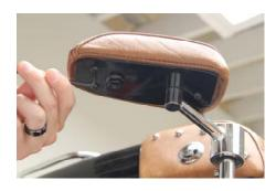
4. If replacing the side panels as well, locate and remove the three bolts mounting the pads to the swivel base using a 4mm Allen wrench.
