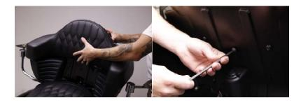
2. Position the armrest in front of the trunk. Use the four supplied 1/4"-20 x 1" Phillips screws and washers to mount the armrest to the trunk. Reconnect the support cables with two of these screws.
