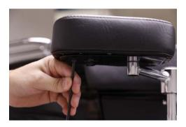
4. If mounting the side pads, position the pads on the swivel bases and, using a 4mm Allen wrench, secure with stock bolts.
