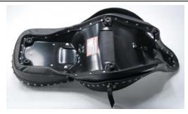
2. Lift rear of seat about 2" and slide seat back and up to remove.
