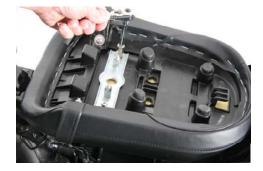
3. Align the latching bracket over the frame locking mechanism and push down on the center of the seat until it clicks, signifying the seat is latched into position. Ensure the bracket is firmly engaged before riding.
