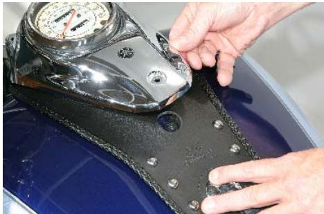
3. Align the small hole in the tank bib with the lower screw hole in the tank. Install and tighten all three Allen screws.
