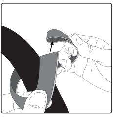
To secure, use the 4 included straps with loop on one side. Pass the strap around a part of the frame or roll cage and pass the strap through the loop creating a noose.
