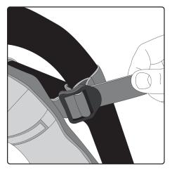
Make sure the strap is locked in place and will not loosen once pulled snug. Repeat on all 4 attachment points.
