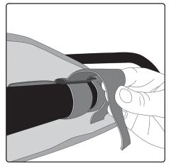
Remove Velcro strap from "D" ring and pass around the roll cage. Re-Insert strap into "D" ring and pull snug before connecting the hook and loop sides of the Velcro. Repeat on all 3 attachment points.
