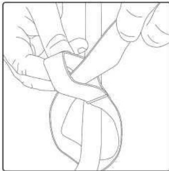
Feed the bladder hose back through the self-fastening closure and remove the bladder.
