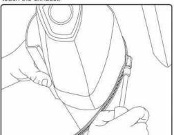
Slide the heat shield and hose clamp over your exhaust and position for optimal protection.
