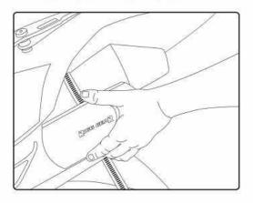
With your mounting location confirmed, use a pair of pliers or metal shears to cut off the excess hose clamp.
