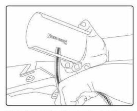
With the heat shield positioned, continue to tighten until snug. Once mounted, double check location and that your Panniers or saddlebags will not touch the exhaust.
