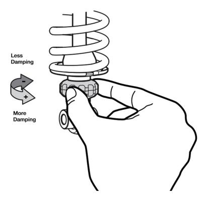
To check it's set correctly, turn in clockwise in the direction of + arrow until it stops, then open 20 clicks. This should be your starting position for rebound. If you want more damping / slower movement, close the rebound in the + direction. If you want less damping / more movement, open the rebound in the – direction.
