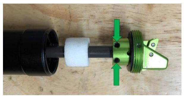
Step 4: Remove ACTUATOR (16) from CARTRIDGE (14)
