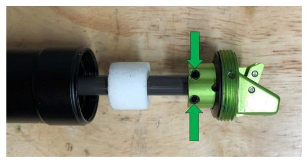
Step 6: Remove ACTUATOR (16) from CARTRIDGE (14)
