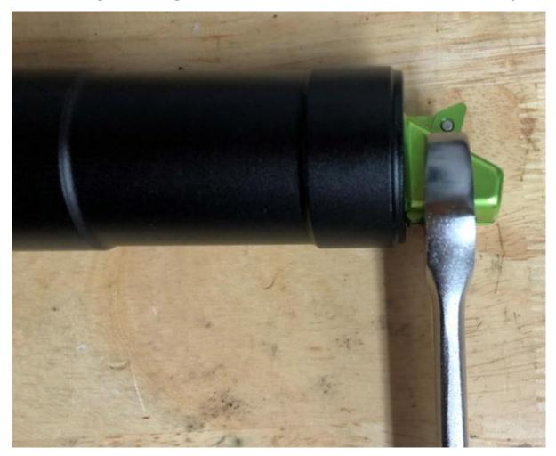
Step 21: Reinstall Seat and UPPER/LOWER CLAMP (2) and (3)
