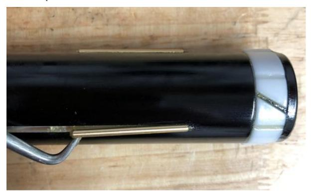
Step 11: Remove BUSHINGS (9) and (11)Remove the upper and lower bushings by hand
