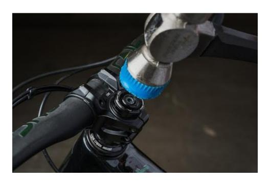
STEP 5: REMOVE YOUR STAR NUT SETTER BOLT AND TOP CAP
