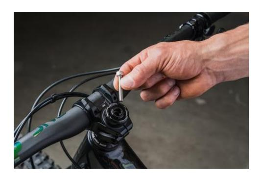
STEP 3: SCREW IN THE STAR NUT SETTER BOLT (LONG BOLT) 10 FULL TURNS.
