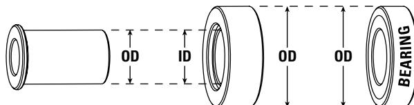
2. **EN Select Bushing** The bushing presses on the outer surface of the bearing to prevent damage. 42 bushings (in 21 sizes) are included, each engraved with its ID, OD and part number. Select bushing with OD that matches OD of bearing and ID that matches OD of pilot and ID of bearing.
