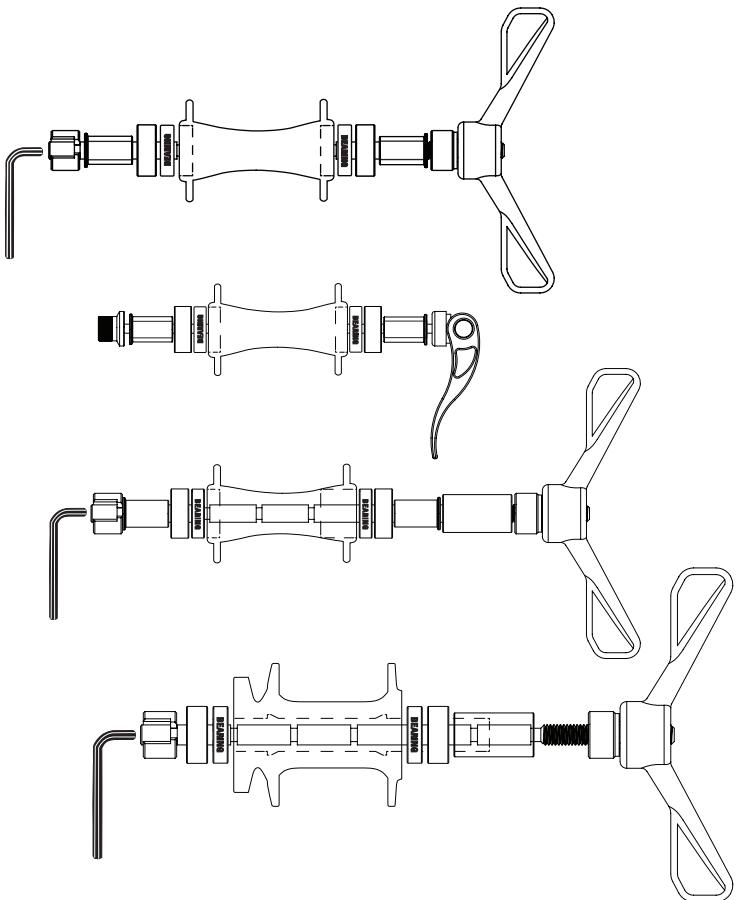
5. **EN Assemble and Press** Assemble hub shell, bearings, bushings, pilots (if needed) and spacers (if needed). Examples of common assemblies are pictured in figures 5a - 5d. Slowly turn handle of press clockwise, making sure components stay aligned. Continue to turn handle until bearings are properly seated in hub. Do not overtighten.
