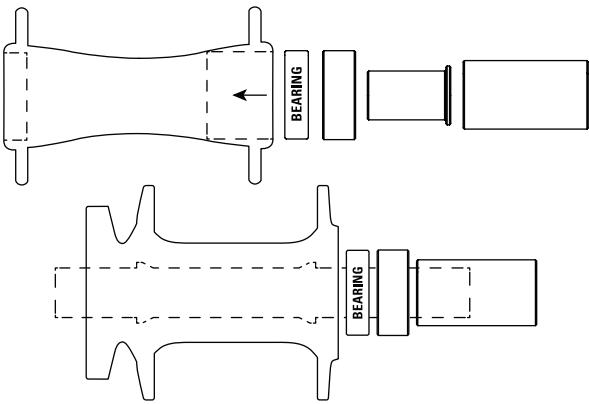
3. **EN Select Spacer (if needed)** 4 spacers are included, each engraved with its ID and part number. The mechanic's judgement is required to determine if a spacer is needed. A spacer is typically used in situations when:
