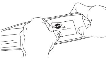
Instructions: Locate cut or tear then clean and dry surrounding surface to promote adhesion of boot. Peel the protective backing from TB-2 and apply, allowing TB-2 to adequately overlap damaged area. Note: The TB-2 is designed for emergency use. A patched tire should be replaced as soon as possible.
