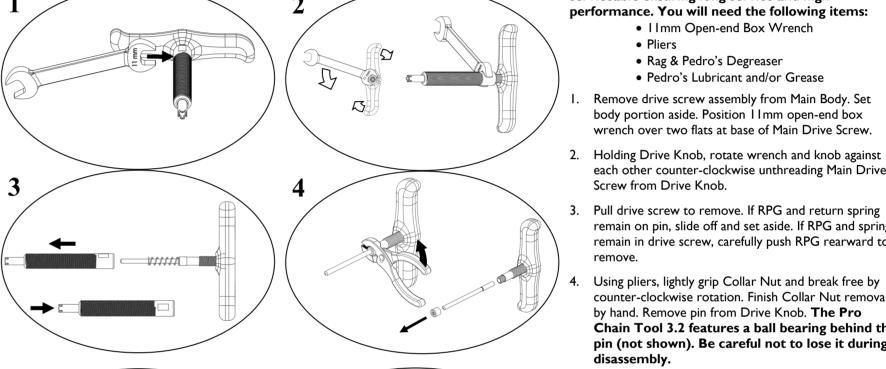
disassembly. 5. With components disassembled, clean any contaminated parts using rag and Pedro's Degreaser. Inspect each part for damage which may impede proper function. Replace if damaged. Lubricate all threaded and sliding parts using a low viscosity lubricant like Pedro's X Dry or Chainj.
