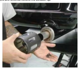
5. With the original exhaust tip removed reinstall the Performance Machine Elite exhaust tip. Align the Performance Machine Logo vertically and make sure the 4 bolt holes line up.
