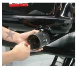
4. Once the four bolts are removed remove the exhaust tip.
