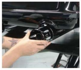
7. Reinstall the four I/4"-20 bolts using red loctite and torque to 7 ft-lbs.
