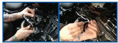
4. On Big Twin & XL models (EXCEPT 08-UP FL) attach the backing plate (4) to the carburetor/throttle body using the supplied I/4"-20 x 5/8" socket head bolts (5) and tighten to 8 ft-lbs. On 2008-UP FL touring models with electronic throttle locate the backing plate (4) to the throttle body using the supplied I/4"-20 x I-I/4" socket head screws. Do not tighten during this step.
