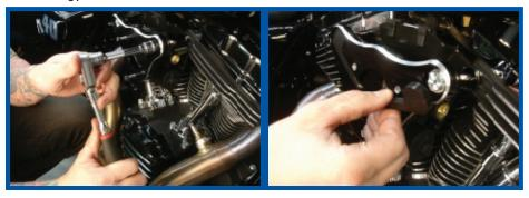
7. On Big Twin and XL models (EXCEPT 08-UP FL) using the supplied  $1/4"-20 \times 3/4"$  socket head bolts (I0) install the secondary plate (8), gasket (II), and complete filter assembly (9) and torque to 8 ft-lbs. On 2008-up FL models with electronic throttle install the secondary plate (8), gasket (II), and complete filter assembly (9) using the  $1/4"-20 \times 1-1/4"$  socket head screws and torque to 8 ft-lbs.
