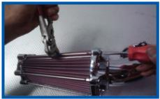
2. Slide the aluminum rear filter cover(I4) off the filter onto the 90degree tube(I2) to expose the hose clamp(I5). Tip: Place masking tape around the 90degree tube(I2) to protect the finish from damage! Loosen the hose clamp to free the filter element(I6).
