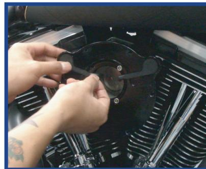
6. Install the secondary plate (11). Install the filter (12) and outer cover (9) at the same time using one 1/4"-3/4" Cap screw (2) to hold the assembly in place. Make sure the round PM logo is clocked to the 9 o'clock position and install the remaining bolts and torque the bolts to 8 ft-lbs.
