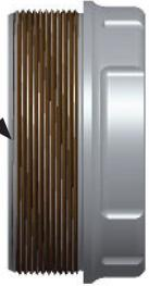
**1.** Apply grease or anti-seize to the frame & BB cup threads
