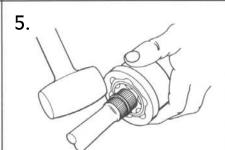
Most other outboard C.V. Joints are held on to the axle shaft with an internal snap ring. These C.V. Joints can be removed by striking the joint face with a mallet.
