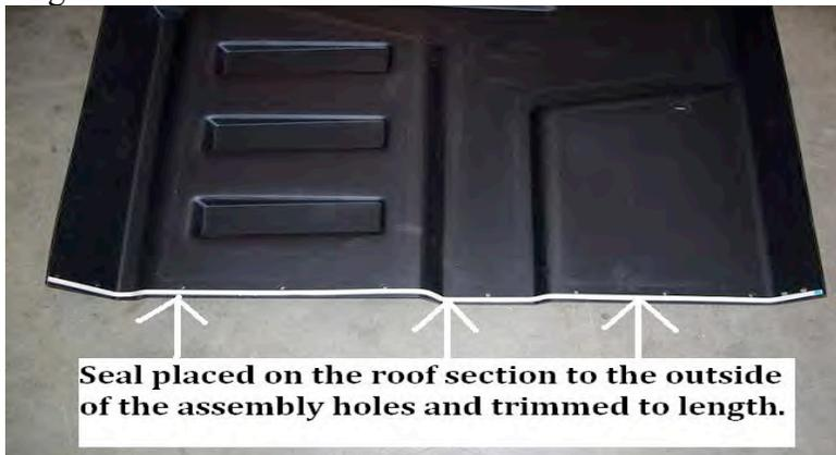
Second place the roof sections together and secure one to the other with the 1/4"-20 x 3/4" long bolts through from the top side with a 1/4" flat washer top and bottom and the 1/4"-20 acorn nuts on bottom side of the roof. This works best starting from the middle and working outward.
