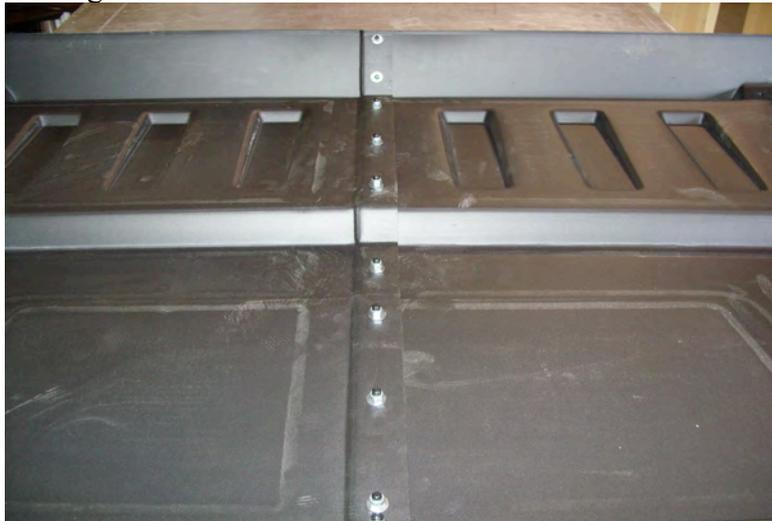
Place the roof on the vehicle and secure with the six P-clamps using the 1/4"-28 x 1" bolt, 1" Fender washer and 1/4"-28 nut.
